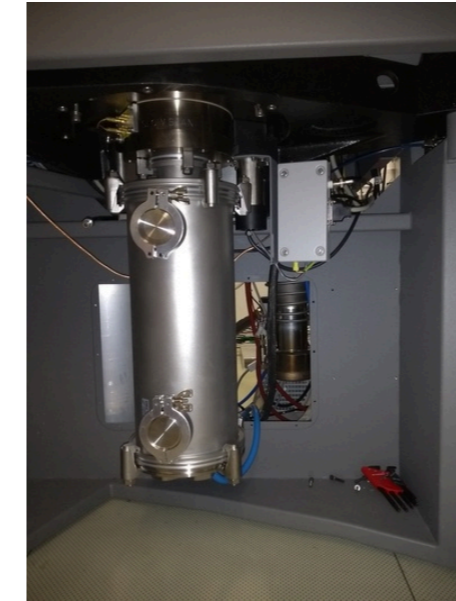
Mounting of the EIGER X 1M with adapter flange
