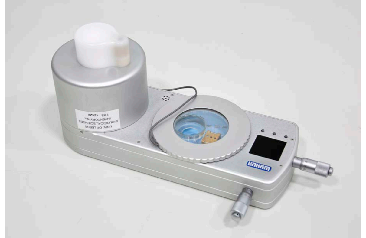
Linkam cryo fluorescence stage (Can be fitted onto Zeiss LSM 880 with Airyscan)
